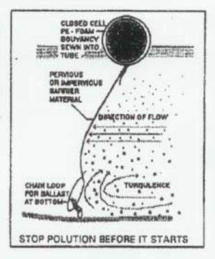
Each turbidity curtain has a floating boom, a barrier fabric or membrane, and a ballasting pocket with or without chain installed as ballast. Ready to deploy units come in 50' or 100'. Accessories allow
